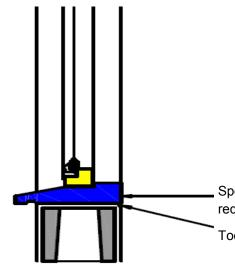
Special weight saving sill profile with integral drip design. No DPC required (cut block to fit sill height)
