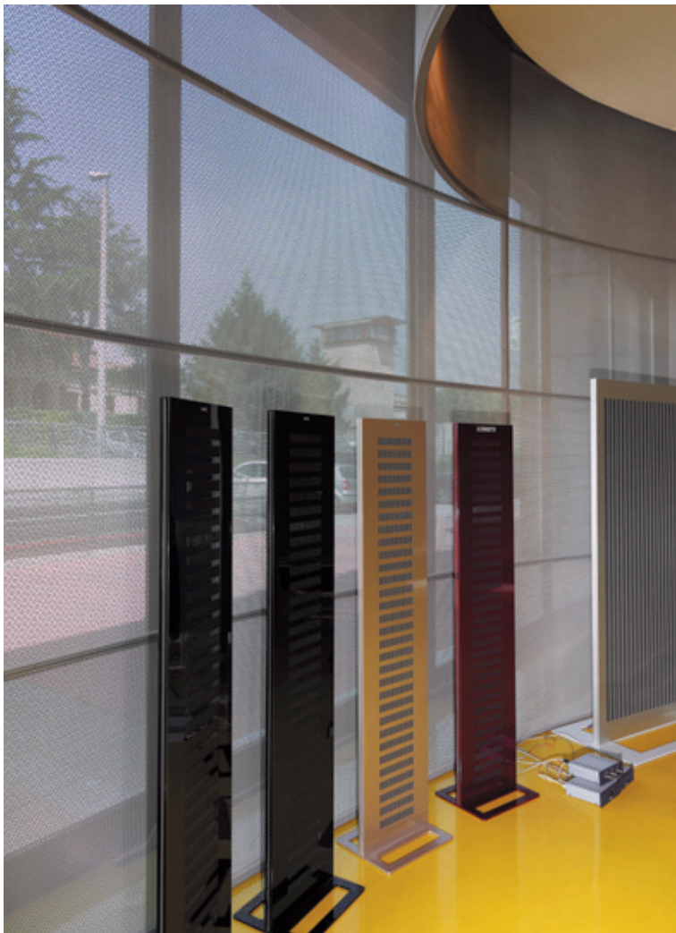
An original elliptical wall divides this large showroom. Made by using two layers of mesh to create the customer reception area. Expanded metal was also used on the stands with rear illumination.
