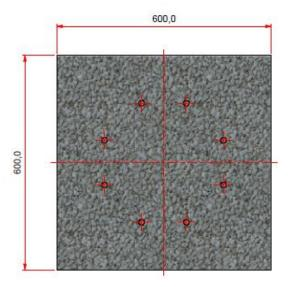
Concrete base to specification at least fck (cube) 300N/mm2 of resistance Base to be flat and level to +/- 5mm over footprint area. Dimensions to be 1400 x 800 x 158 deep min. (Units in mm)
