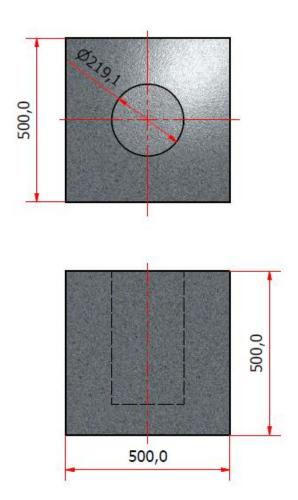
Concrete base to specification at least fck (cube) 300N/mm2 of resistance Base to be flat and level to +/- 5mm over footprint area. Dimensions to be 500 x 500 x 500 deep min. (Units in mm)
