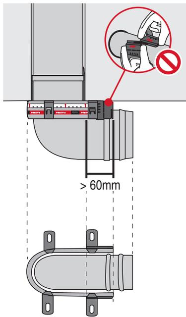
**Installation overview:** To the recommended length of the diameter it's necessary to add 120mm. The reason for that is that the hooks of the closure plates (Which are absolutely crucial for this application) need to be fixed in the base material and with a safe distance from the final of the opening. The collar doesn't need to be closed for this application; it's installed with a U-Shape around the collar.
