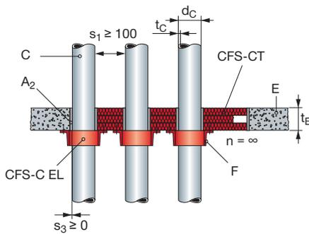
**Description:** Hilti Firestop Collar endless CFS-C EL can be used to firestop plastic pipes penetrating a wall seal made of mineral wool.
