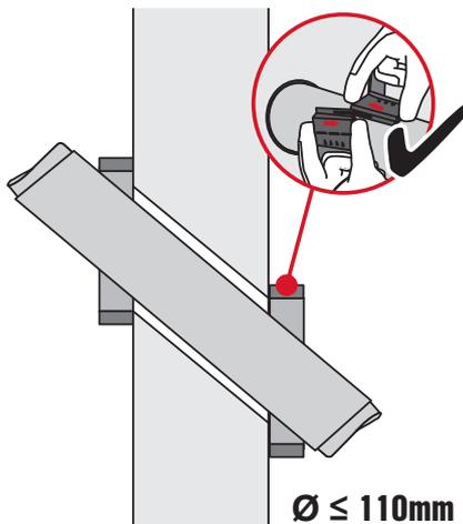
**Installation overview:** For this application it's necessary to measure the length of the Hilti Firestop Collar Endless CFS-C EL directly on the pipe. It's crucial that there is no space between the Collar and the pipe. The recommended number of hooks is shown below.
