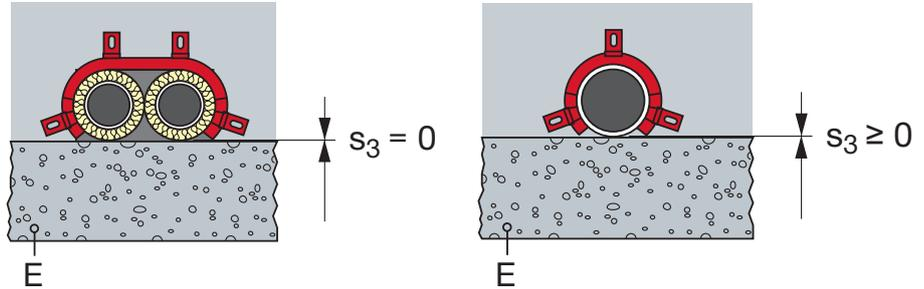
**Installation overview:** The length should be measured directly on the penetrating pipes. It's very important that the distance between two hooks is never bigger than 150 mm.
