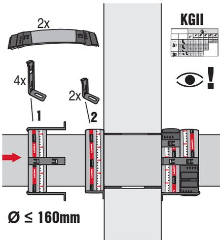
**Installation overview:** It's necessary to cut two identical pieces with the recommend length (See table below) and install the closure plates at each end.
