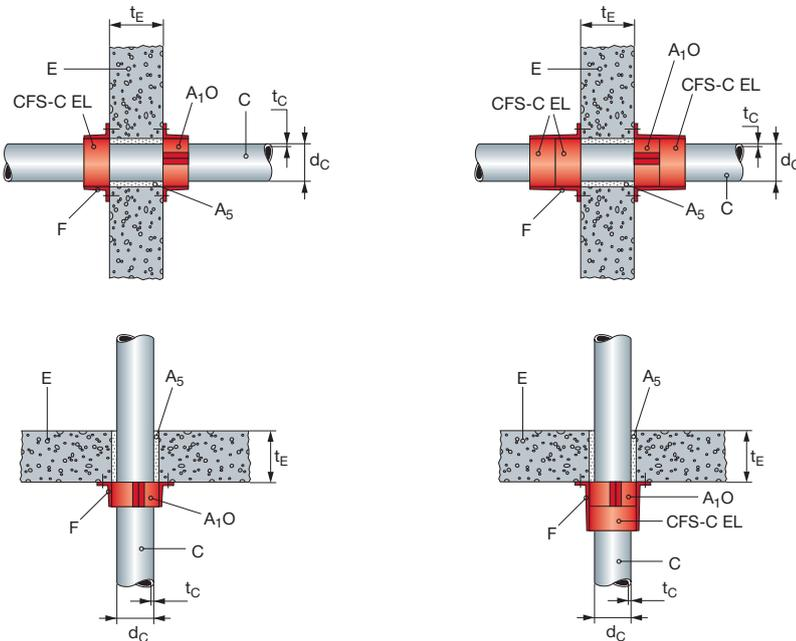
Pipes containing oddments ( $A_{10}$ ) in application group 1 and 2 in wall and floor penetration
