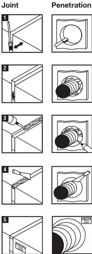
Clean opening. Surfaces to which CFS-S ACR will be applied should be dry, cleaned of loose debris, dirt, oil, wax and grease. Use wire brushing for cleaning.
