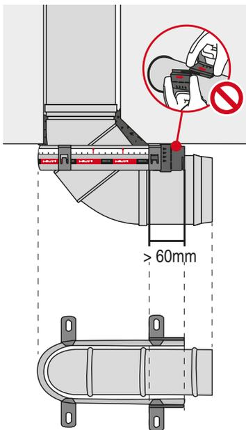
**Installation overview:** To the recommended length of the diameter it's necessary to add 120mm. The reason for that is that the hooks of the closure plates (Which are absolutely crucial for this application) need to be fixed in the base material and with a safe distance from the final of the opening. The collar doesn't need to be close for this application; it's installed with a U-Shape around the collar.
