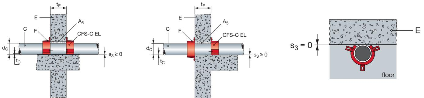
**Installation overview:** Measure the length needed for the pipe diameter directly on the penetration. It has to cover more than 3/4 of the total perimeter of the pipe.
