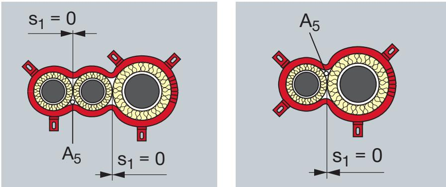
**Installation overview:** The length should be measured directly on the penetrating pipes. It's very important that the distance between two hooks is never bigger than 150 mm.
