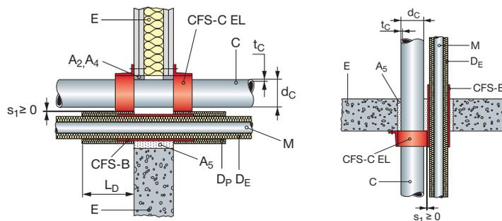
In floor application ( $t_E > 150 \text{ mm}$ ) there is no need for an additional protect insulation  $D_P$ .
