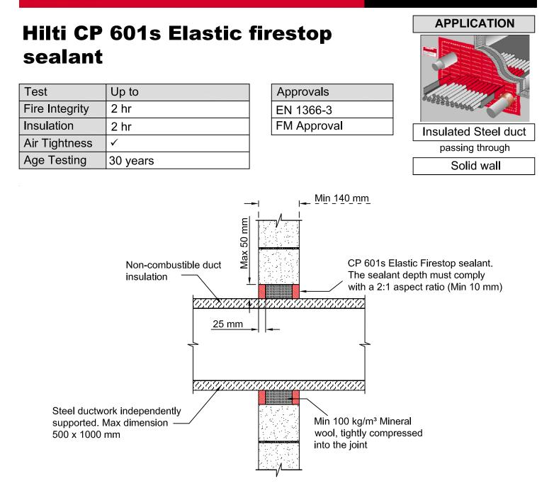
The performance of the Fire Rated Duct system must be proven by test to be capable of achieving the required fire rating of the seal system - up to 120 minutes Fire Performance.
