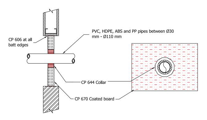
The CP 670 coated board should be installed tightly around the service pipe. CP 606 Intumescent mastic must be used at all batt edges in accordance with the installation guidelines.
