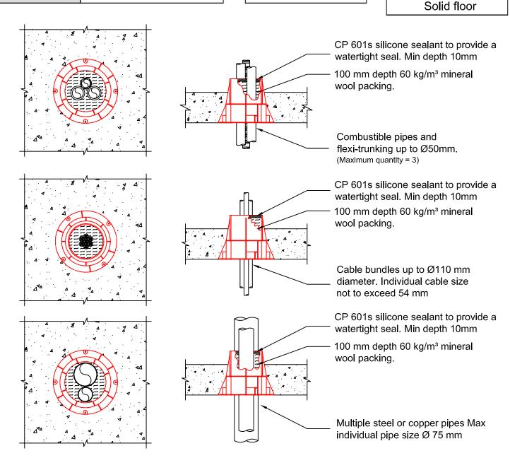
All services to be supported either side of the seal system. Mineral wool insulation not to extend to the intumescent collar at the base of the device, which might impair its performance.
