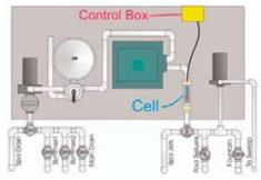
Figure 11.2 – A typical salt water circulation and treatment system4.
