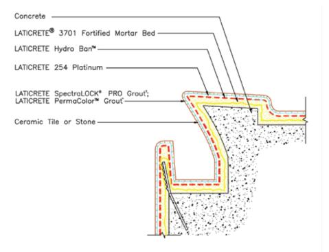
Note: Slurry Bond Coat of LATICRETE 254 Platinum is required under the mortar bed at all horizontal surfaces.
