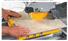
Figure 6.7 – A commercial grade wet saw is ideal for cutting all types of tile and stone in swimming pool, fountain or water feature applications.
