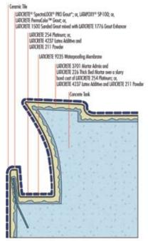
DETAIL AT SWIMMING POOL GUTTER AND POOL DECK
