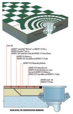
Figure 7.21 – Thick Bed Floor / Waterproofing System with drain detailing.
