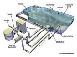
Figure 4.5 – Cut away view of a typical pool pump and filtration system.<sup>7</sup>
