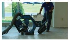
Figure 6.3 – Shot-blasting is ideal for areas outside of pool tanks and water features and for areas where access by the equipment is not an issue.
