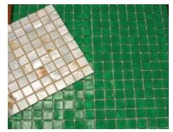
Figure 5.4 – Two examples of paper-face mounted glass mosaic tile.
