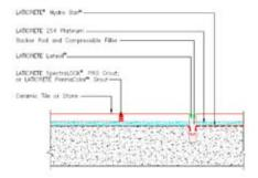
Case Study 6 – Movement joints are also included in the pre-treated areas. The waterproofing membrane is looped down into the movement joint (to accommodate any potential movement). The waterproofing membrane must be given enough "slack" when looped into the joint to accommodate the anticipated movement. The waterproofing membrane is then lapped onto the concrete / mortar bed joint flanks and horizontal areas by at least 2 – 4" (50 – 100 mm) to receive the main waterproofing membrane treatment.
