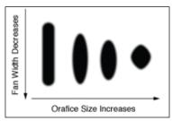
Figure 6.18 – The example demonstrates the spray pattern of new and worn spray tips. As wear occurs, the pattern size decreases and the orifice size increases. As a rule of thumb, it is best to replace the spray tips after spraying 30–45 gallons (114–171 liters) of LATICRETE Hydro Ban $^{\rm TM}$ .
