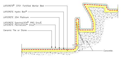
Note: Slurry Bond Coat of LATICRETE 254 Platinum is required under the mortar bed at all horizontal surfaces.
