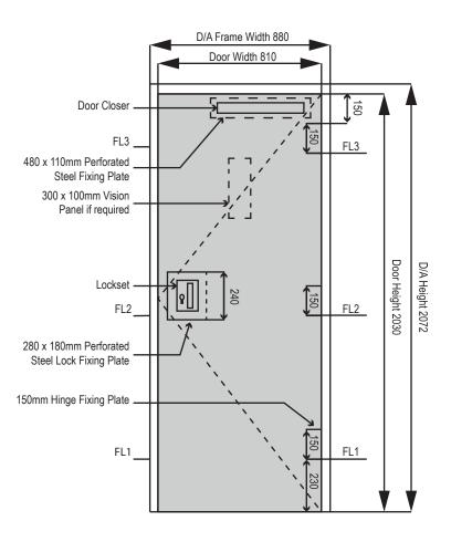
When ordering steel door frames or doorsets it is important to nominate the handing, and state correct reveal height and width required.
