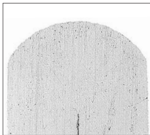
Fig. 4: Metallographic cross section of a flexural test piece after a 180° fold, without an intermediate layer, parallel to rolling direction
