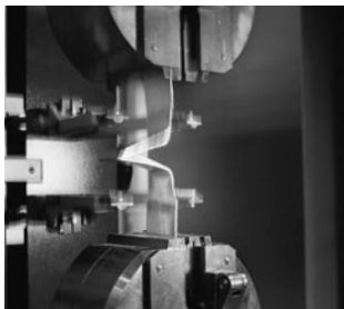
Fig. 3: Tensile seam test in the RHEIN-ZINK-Quality Control Dept.
