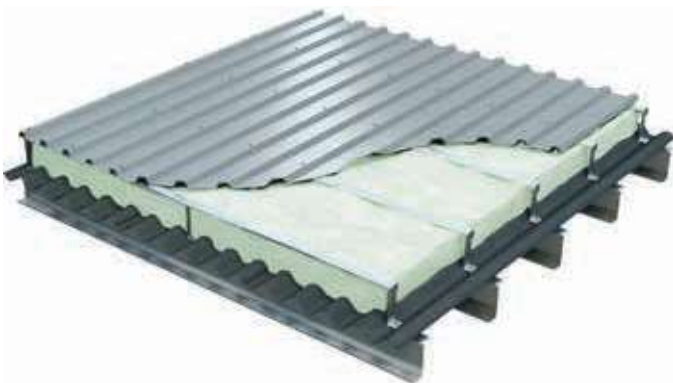
Spacer system used to over roof an existing asbestos roof with Saftherm polyester blanket insulation in the void created.
