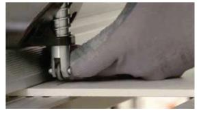
When the cut has been made, move the slab until the incision line sticks out 10 cm from the workbench.
