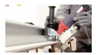
Manual traction devices are available in order to make a finishing cut at 45° and thus enable special applications of the material.
