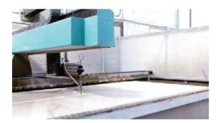
Water-jet cutting can be used either to carry out both linear cuts and holes. Please note that in case the supporting grid is not optimum, the use of a rigid carton placed underneath reduces vibrations, thus facilitating the cutting procedures.
