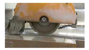
For the processing: marble and granite equipment can be used, whereas the diamond blades shall be specific for porcelain stoneware. Finally, we recommend the use of adequate equipment to handle the slabs.
