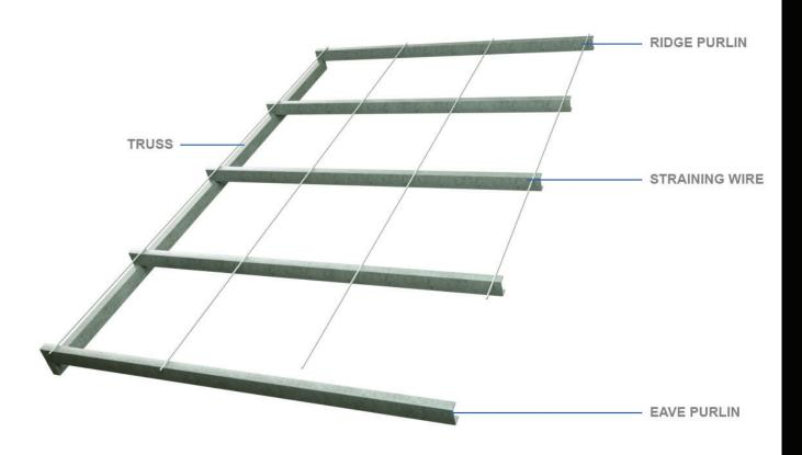
Fix PVC coated straining wire from the top apex purlin, over intermediate purlins to the bottom eave purlin at 383 mm centers. First straining wire to be fixed 50 mm away from gable end. Evenly tension all wire ensuring that cut ends face downwards.
