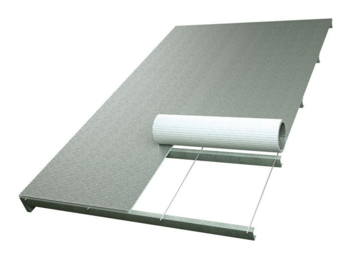
Lay Alucushion® / Bubblefoil® FR over the straining wires ensuring that it is squared off. Fix to apex purlin using double-sided tape. Evenly tension material and fix to eave purlin again using double-side tape.
