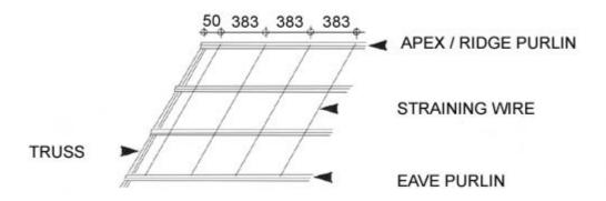
• Lay Alucushion® / Bubblefoil® FR over the straining wires ensuring that it is squared off. Fix to apex purlin using double-sided tape. Evenly tension material and fix to eave purlin again using double-side tape.
