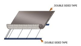
Roll ALUBUBBLE® down the slope of the roof and cut to length with an additional 200mm of material to use as a grip for tensioning the material. Fix ALUBUBBLE® over the straining wires and ensure that it is laid square to the building. Attach ALUBUBBLE® to the eaves purlin using good quality double sided adhesive tape of either 24mm or 48mm width. Firmly grip the top end of the material and pull to tension the ALUBUBBLE® and attach to the apex purlin again using double sided tape.
