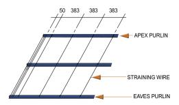
Fix PVC coated straining wire by passing it through 5mm holes drilled in the top faces of the apex/top purlin and the eaves/bottom purlin at 383mm centres. The wire to pass over the intermediate purlins. The first straining wire to be fixed 50mm away from gable end. Evenly tension all wire ensuring that cut ends face downwards.
