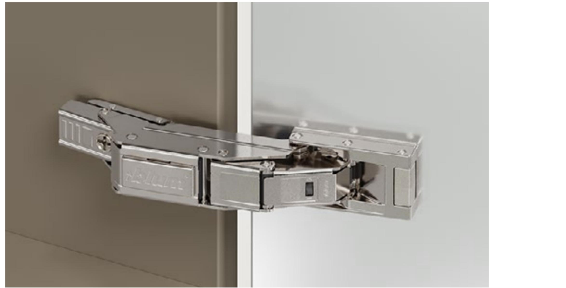
Hinge without door protrusion. Adhesion plate is UV bonded onto glass (no glass drilling necessary)
