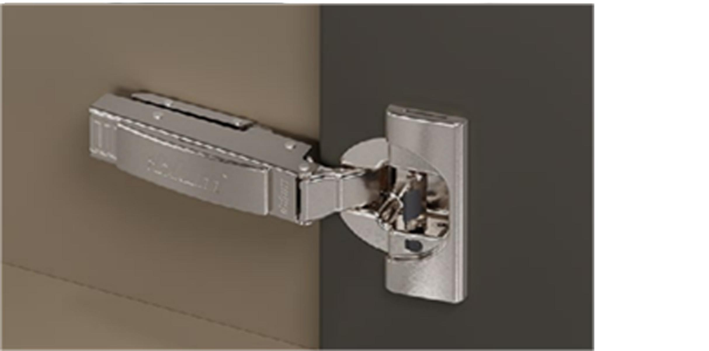
Hinge for standard applications. Integrated BLUMOTION. Low boss drilling depth for furniture doors with a thickness of 35 mm.
