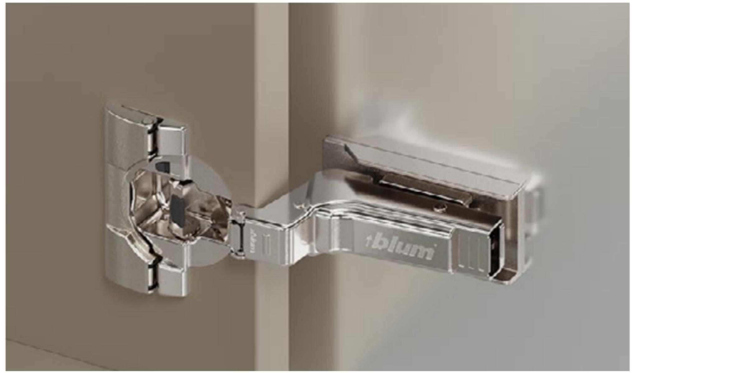
Hinge for mirror fronts. 95° opening angle. Integrated BLUMOTION soft-close system for soft and effortless closing action (with deactivation). Mounting plate is glued on to the front, without glass drilling, boss drilling on the cabinet.
