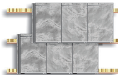
Tiles must be laid broken-bond and mechanically fixed according to specifications movement.
