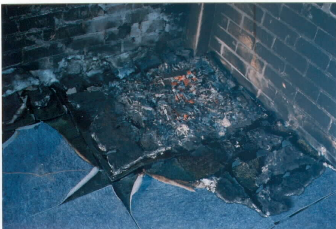
Figure 12: Close-up view of remnants of crib Note limit of flame spread
