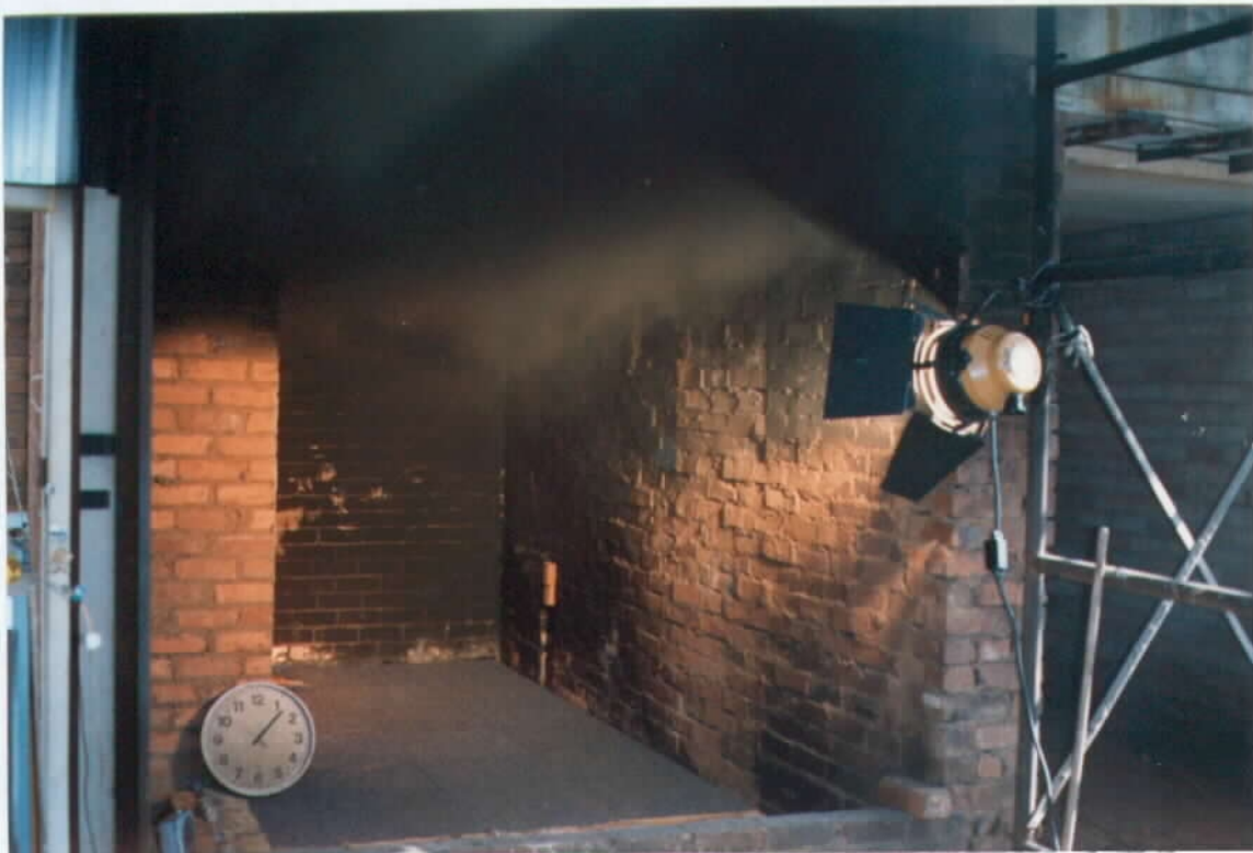
Figure 7: 7 minutes after ignition Note buoyant smoke cloud
