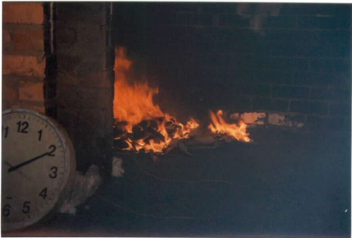
Figure 8: 10 minutes after ignition Note small extent of flame spread
