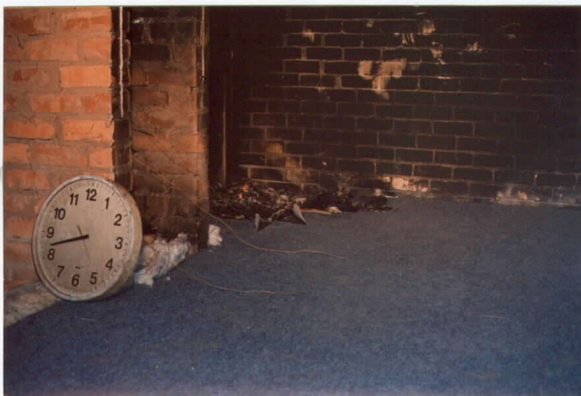
Figure 11: Carpet extinguished - ignition source still glowing
