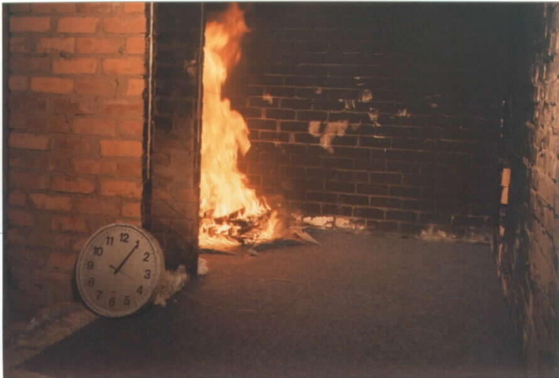
Figure 6: Carpet starting to burn 05:25 minutes after ignition
