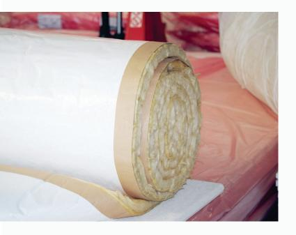
For industrial over-purlin applications the faced Starlite® is manufactured to the required length within the standard limitations (500mm increments) and laid over-purlin directly below the roof sheet.
