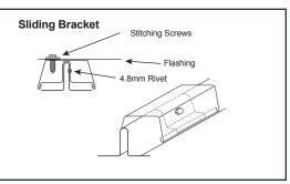
\* When sheet lengths are over 30m (20m for Aluminium) flashings must be fixed to sheets using sliding brackets.
