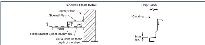
\* When sheet lengths are over 30m (20m for aluminium) flashings must be fixed to sheets using sliding brackets.
