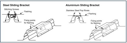
When sheet lengths are over 30m (20m for Aluminium) flashings must be fixed to sheets using sliding brackets.
