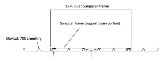
Sliding brackets to be used on side sheets when length exceeds 30m for steel sheets & 20m for aluminium sheets. For shorter sheets use S10 brackets.
