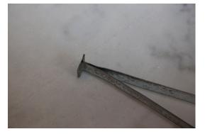
Tie Strap – feed both legs through hole in underslung frame
