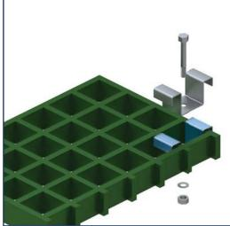
The rib of the sheeting determines the position required for the M-Clamp. In order to align correctly it is necessary to cut out an appropriate cross member, and also notch out the two adjacent cross members to clear the bracket lips.
