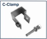
C-clamps are designed to tie two neighboured panels of molded fiberglass gratings together. This helps to minimize differential deflections when their joints fall between supports. The installation is from the top side of the fiberglass grating walkway.
