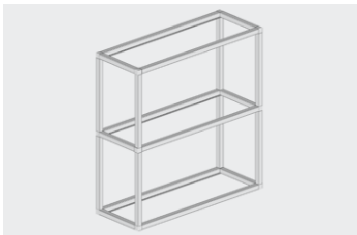
Top cabinet vCUBE frame: for 3 timber shelves on the top, bottom and middle
