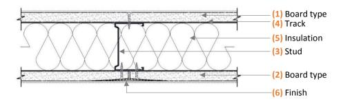
For system heights exceeding 4200 mm, use Gypframe® UltraSteel® Deep Track for both floor and head tracks. For systems with expected deflection of >10 mm and <4200 mm height, use Gypframe® UltraSteel® Deep Track for head tracks only.
