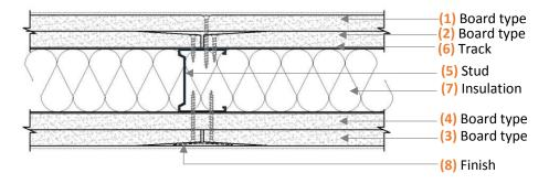
For system heights exceeding 4200 mm, use Gypframe® UltraSteel® Deep Track for both floor and head tracks. For systems with expected deflection of >10 mm and <4200 mm height, use Gypframe® UltraSteel® Deep Track for head tracks only.
