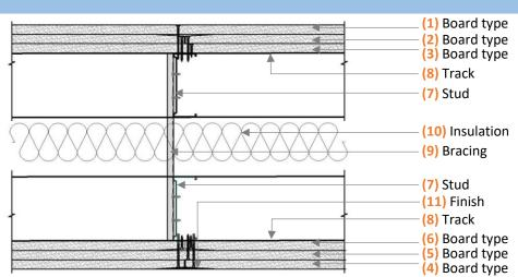
For system heights exceeding 4200 mm, use Gypframe® UltraSteel® Deep Track for both floor and head tracks. For systems with expected deflection of >10 mm and <4200 mm height, use Gypframe® UltraSteel® Deep Track for head tracks only.
