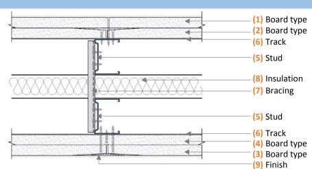
For system heights exceeding 4200 mm, use Gypframe® UltraSteel® Deep Track for both floor and head tracks. For systems with expected deflection of >10 mm and <4200 mm height, use Gypframe® UltraSteel® Deep Track for head tracks only.
