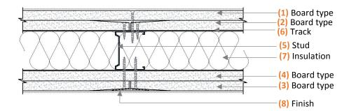
For system heights exceeding 4200 mm, use Gypframe® UltraSteel® Deep Track for both floor and head tracks. For systems with expected deflection of >10 mm and <4200 mm height, use Gypframe® UltraSteel® Deep Track for head tracks only.
