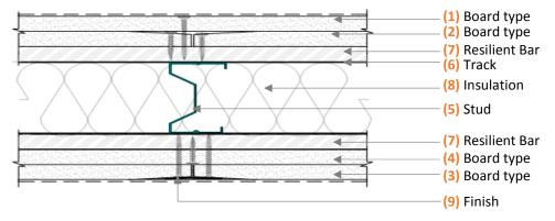
For system heights exceeding 4200 mm, use Gypframe® UltraSteel® Deep Track for both floor and head tracks. For systems with expected deflection of >10 mm and <4200 mm height, use Gypframe® UltraSteel® Deep Track for head tracks only.
