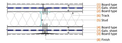
For system heights exceeding 4200 mm, use Gypframe® UltraSteel® Deep Track for both floor and head tracks. For systems with expected deflection of >10 mm and <4200 mm height, use Gypframe® UltraSteel® Deep Track for head tracks only.
