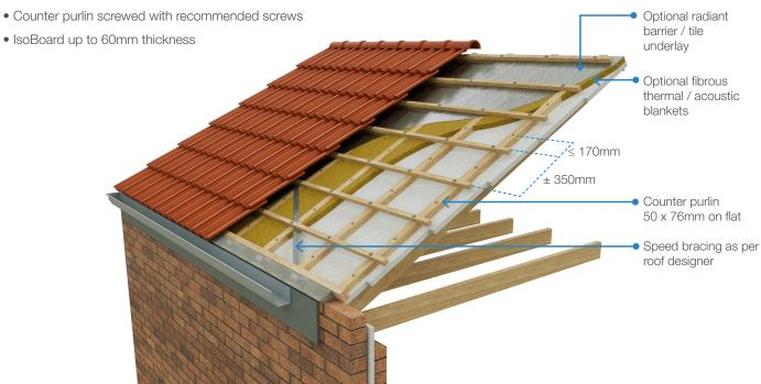
Truss vertical and in plane bracing shall comply with SANS 10243. For tiled trussed roof system an in-plane braced bay shall connect at least three adjacent trusses with metal brace.
