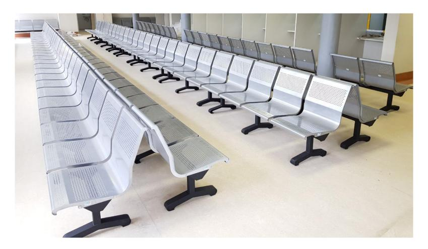
The Rodlin Design Versa seating features a one-piece seat shell manufactured in either 430 brushed stainless steel at 1.2mm thickness or 2.0mm mild steel, available in perforated or non-perforated options. The seat shell incorporates integrated 5mm rigid spines designed to prevent flexing or bending of the backrest under pressure.
