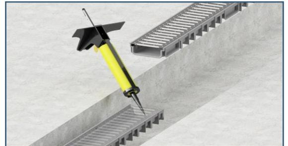
2. Apply the sealant on the of the connection area (male/female) and install the channels.
