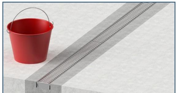
4. Finally fill the trench with concrete in order to completely fill and close all the spaces left free around the channels.
