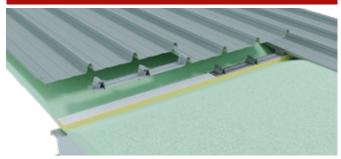
Saftherm™ polyester blanket insulation compressed with an insulating packer. The concealed fix clip is fastened through the packer into the purlin.
