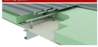
Spacer system in conjunction with a liner sheet to create a void for the Saftherm™ polyester blanket insulation.
