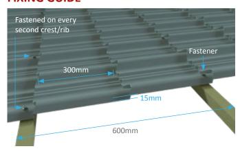
Versatile® is pierce fixed to steel or timber supports. This means that fasteners pass through the sheeting. To maximise water tightness, always place the roof fastener through the crest of the sheeting. Always drive the fastener perpendicular to the sheeting and in the centre of the crest. A standard lap is 1 flute. It is generally considered good practice to use fasteners alongside laps. It's further recommended that every rib is fixed at the eaves, ridges and the apex of the roof.
