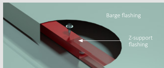
Newlok™ Z-support flashings for longitudinal flashings.
