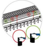
Image detailing how the two fixing systems anchor the grates to the channels.
