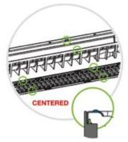
The channels contain protrusions to assist in anchoring the grates to the channels. No external elements such as screws are required.
