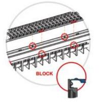
The channels contain pivots to assist in centering the grates to the channels. The pivots further lock the grating into position to keep them centered and stabilized.
