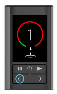
The amount of green encircling the flow rate selected will increase or decrease as the flow rate is, respectively, adjusted upwards or downwards.
