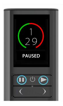
The Triton Xerophyte Controller Unit provides default function and display re-configuration options to personalize your shower experience. These can be accessed and activated while the Controller Unit is in sleep mode. To activate the Configure (or Configuration) Menu, press and hold down at the same time both the Start/Stop Button ( ( ) ) and the Flow Decrease Button ( ( ) for 3 seconds.
